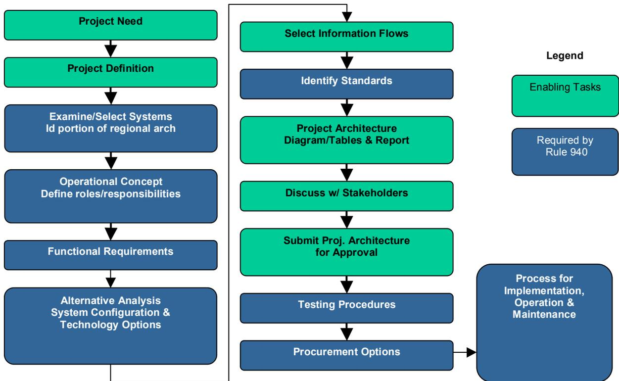
**Figure 3: Process to develop Detailed Project Architecture (After Funding Approval)**
